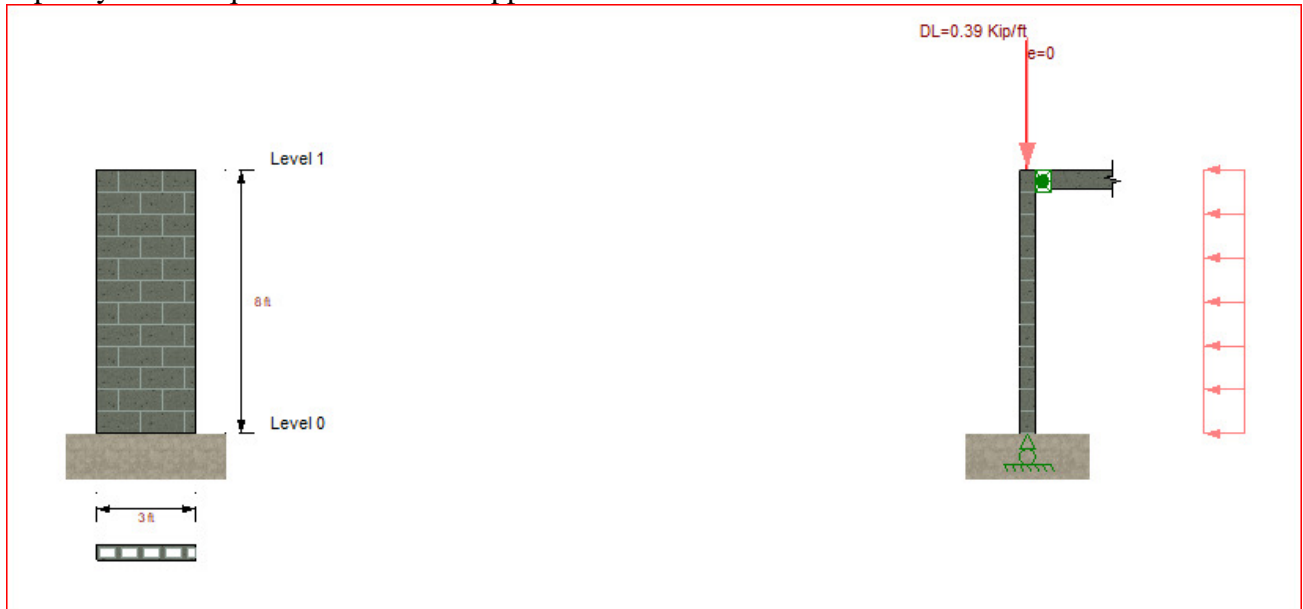
Figure 6: 2D View of Ram Elements Design Model of Outer CMU Wall
