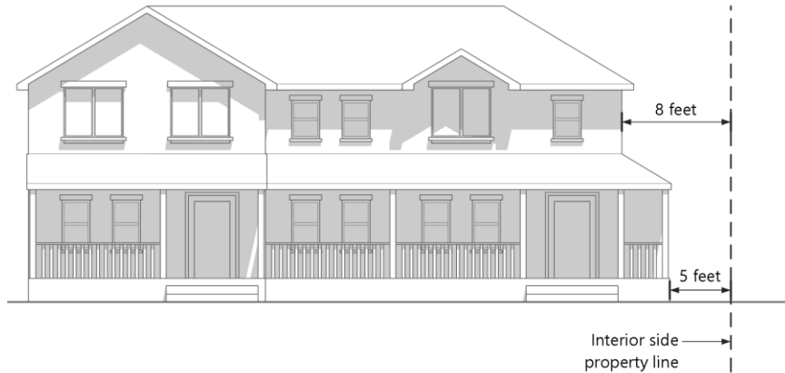
Figure 4.8. Partial Two-Story Structure with Additional Setbacks
