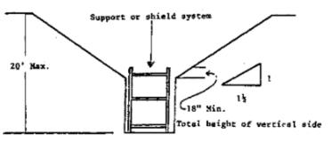
BENCHING – Is a method of protecting workers from cave-ins by excavating the sides of an excavation to form one or a series of horizontal levels or steps, usually with vertical or near vertical surfaces between levels. BENCHING CANNOT BE DONE IN TYPE C SOIL.
